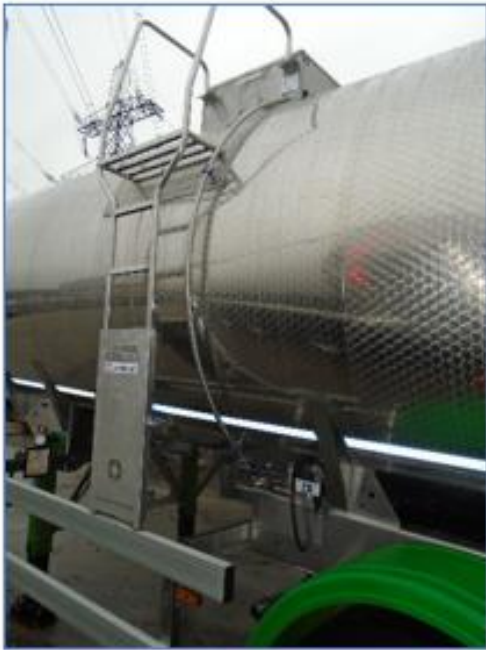
Security cable system secured to N/S Bogie Rail, along with ladder restriction.
