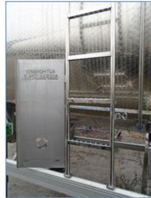
Ladder restriction open
